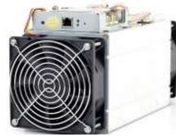
Specialized HW for hashing (ASIC)
